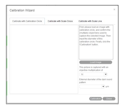
Select the different tabs to display the corresponding panels. Follow the instructions outlined in the corresponding panel to calibrate.
