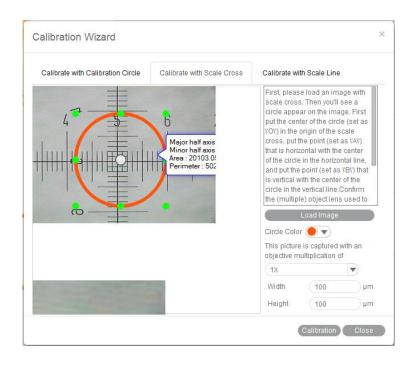
The Save Sign dialog box will display when the Calibration button is selected. Input a Sign Name by clicking the corresponding objective lens from the list at the left of the dialog box.
